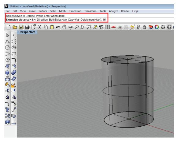
There are many ways create a cylindrical shape. The loft and extrude commands are very common commands in 3D construction. The loft command requires 2 or more closed curves, while the extrude command only requires one.
