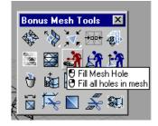
Select gap edge and it will be automatically filled with mesh polygons. No naked edges.
