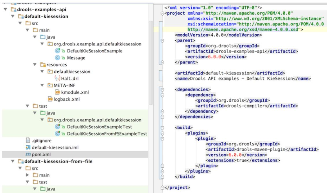
**Figure 4.2. Example project layout and Maven POM**
