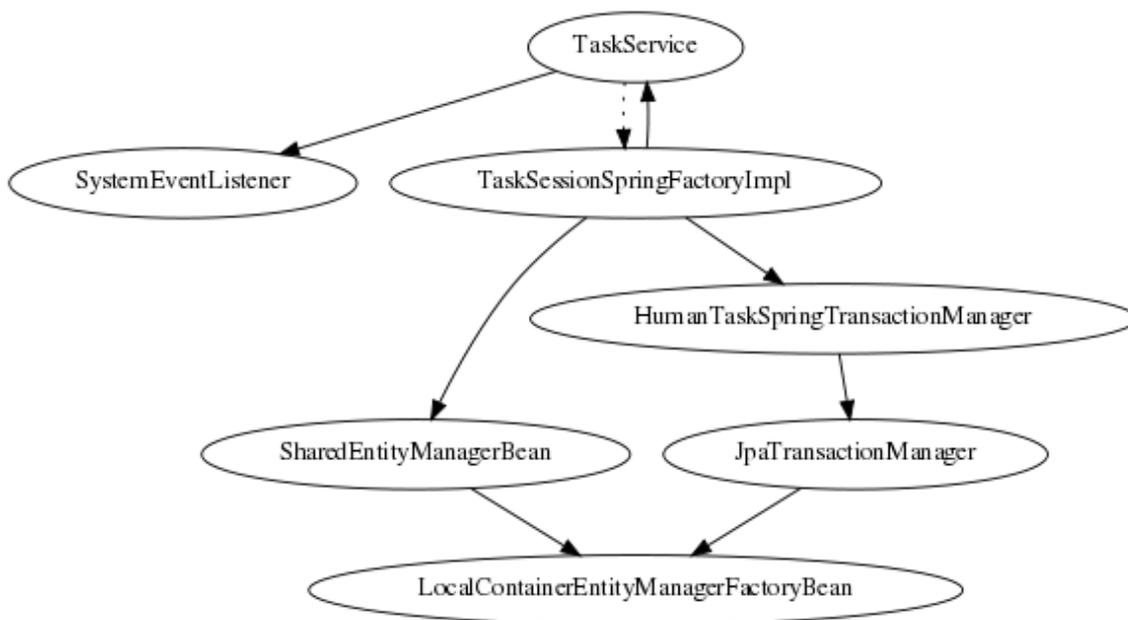
**Figure 11.3. Spring Human Task integration injection dependencies**
