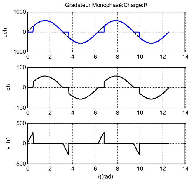
2. Tension efficace :  $U_R = V_m \cdot \sqrt{1 - \frac{\alpha}{\pi} + \frac{\sin(2\alpha)}{2\pi}} = 400 \cdot \sqrt{1 - \frac{1}{6} + \frac{\sqrt{3}}{4\pi}} = 394V$
