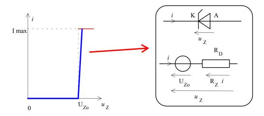
$\begin{array}{lll} \textbf{diode passante} & i \geq 0 & u_Z = U_{Zo} + R_Z \, i & sch\'{e}ma \, \'{e}quivalent \\ \textbf{diode bloqu\'{e}e} & i = 0 & u_Z \leq U_{Zo} & interrupteur ouvert \\ \end{array}$
