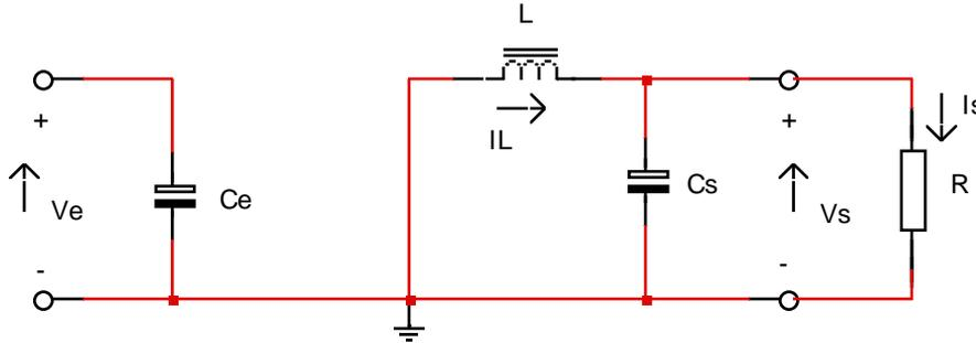
$$-V_s = L \frac{di}{dt} \quad \text{ou} \quad V_s = -L \frac{di}{dt}$$
