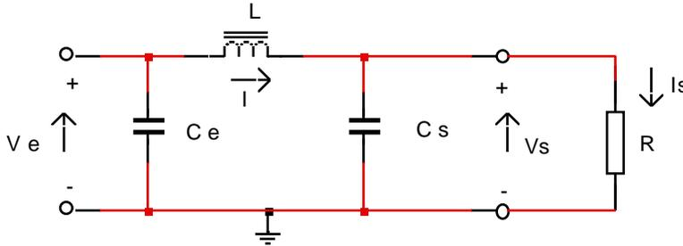
$$V_e - V_s = L \frac{di}{dt} \quad \text{ou} \quad V_s - V_e = -L \frac{di}{dt}$$
