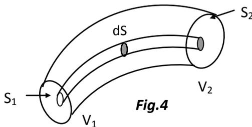
$$\text{On a : } V_1 - V_2 = \int_1^2 \vec{E} \cdot d\vec{\ell} = \int_1^2 \frac{\vec{j}}{\gamma} \cdot d\vec{\ell} = \int_1^2 \frac{j}{\gamma} d\ell$$
