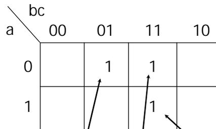
$$f(a,b,c) = \overline{a}.\overline{b}.c + \overline{a}.b.c + a.b.c$$
