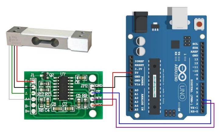
Load Cell Interface with Arduino
