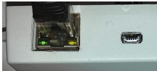
Photo on the right shows the Arduino server box running on POE with USB cable unplugged.
