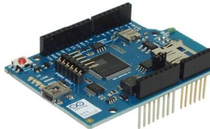
Figure 6 : Shield WIFI Arduino
