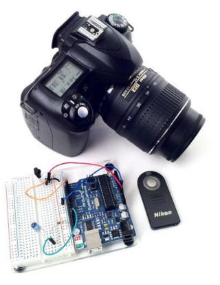
The camera we'll be using has an IR remote you can use to set it off (most higher-end cameras have these).
