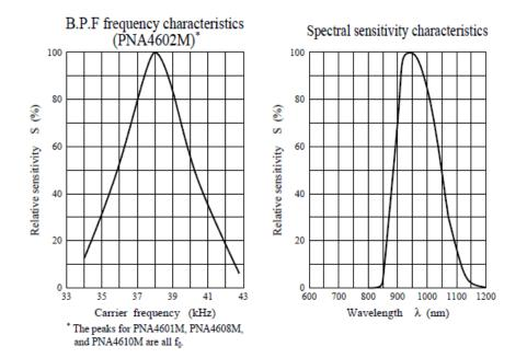
As you can see from these datasheet graphs, the peak frequency detection is at **38 KHz** and the peak LED color is **940 nm**. You can use from about 35 KHz to 41 KHz but the sensitivity will drop off so that it wont detect as well from afar. Likewise, you can use 850 to 1100 nm LEDs but they wont work as well as 900 to 1000nm so make sure to get matching LEDs! Check the datasheet for your IR LED to verify the wavelength.
