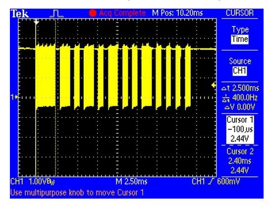
Basically we see pulses or IR signal. the yellow 'blocks' are when the IR LED is transmitting and when there is only a line, the IR LED is off. (Note that the voltage being at 3VDC is just because of the way I hooked up the sensor, if I had swapped the pullup for a pulldown it would be at ground.)
