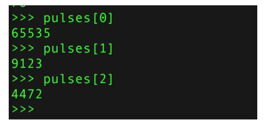
Each duration is the time in milliseconds that the pulse was at a specific logic level. The very first pulse is a maximum value of 65535 because it represents the amount of time the sensor was waiting for the pulse to start (i.e. how long it was in the default high logic level idle state). Just like with the Arduino code on the previous page you can ignore this first value.
