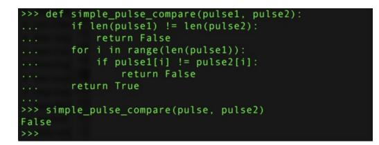
Oh no, the comparison failed and returned false! What happened, wasn't the same button pressed? It turns out the timing between pulses can vary in small ways. If you look at the individual pulse lengths of each array you'll see they're close but not exactly the same. If you compare raw pulses you need to add a 'fuzzyness' that compares values that are close but not exactly the same.
