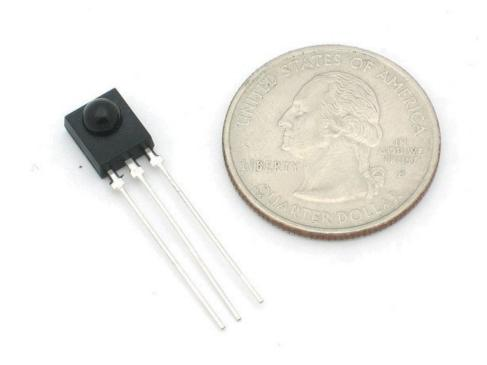
IR detectors are little microchips with a photocell that are tuned to listen to infrared light. They are almost always used for remote control detection - every TV and DVD player has one of these in the front to listen for the IR signal from the clicker. Inside the remote control is a matching IR LED, which emits IR pulses to tell the TV to turn on, off or change channels. IR light is not visible to the human eye, which means it takes a little more work to test a setup.
