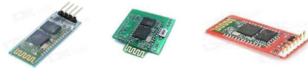
*Figure II.11 Type de modules Bluetooth*
